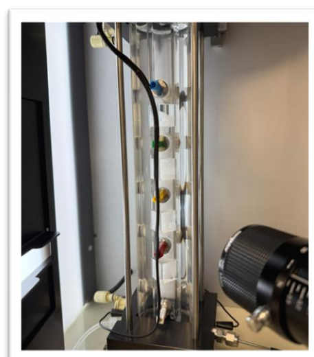
FOAMSCAN™ equipped with the small diameter Double-walled cylindrical glass measuring tube and the gas sparging base
